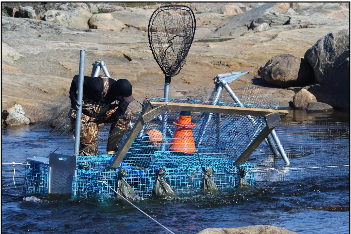
Figure 1. Counting fence and holding cage used to monitor Arctic Char during its upstream migration in August and September 2018 in the Five Mile Inlet system north of Inukjuak, Nunavik.
